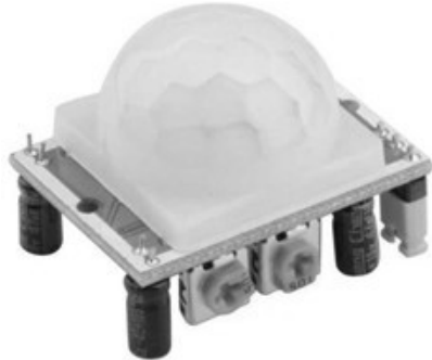
Figure 10: HC-SR501 infrared motion sensor
