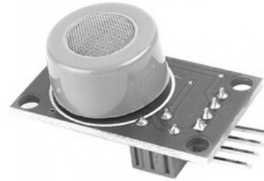
Figure 7: Sensor of combustible gases and carbon monoxide MQ-9
